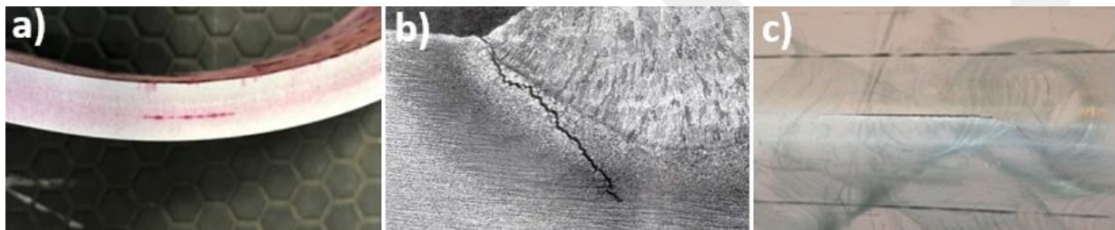
Figure 1.5 The cracks thought to be caused by hydrogen during production process a) after laser cutting, b) after welding, c) after bending process
