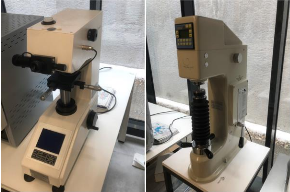
Figure 4.10 Microhardness (on the left) and macro hardness (on the right) test devices
