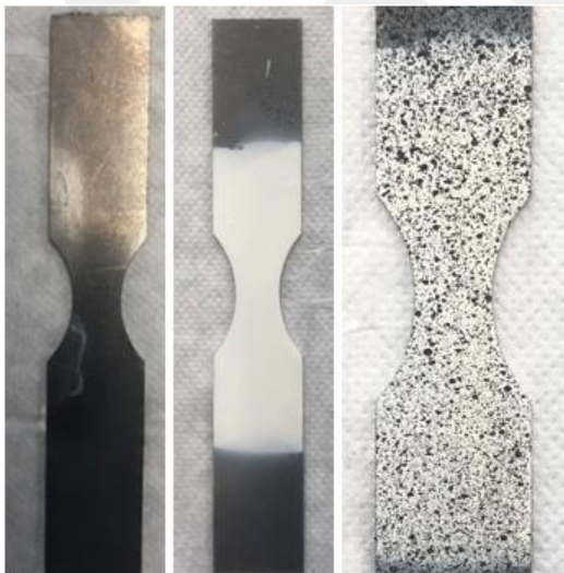
Figure 4.31 A speckle pattern application with tensile test specimen
