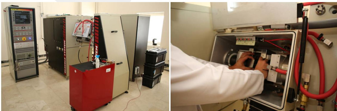
Figure 4.12 Gleeble 3500 mechanical testing system
