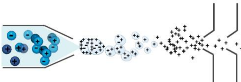
Figure 1.7 Illustration of electrospray ionization.
