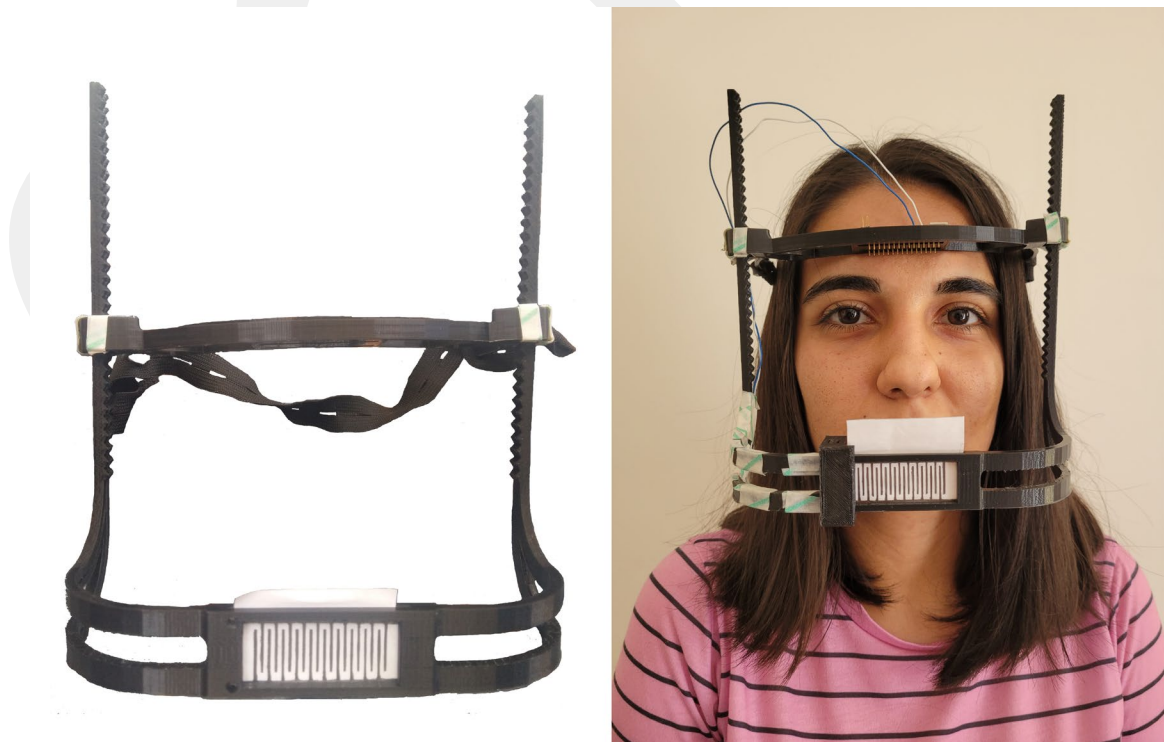
Figure 3.32 A) The head mask for the sensor. B) Usage example of the head mask
