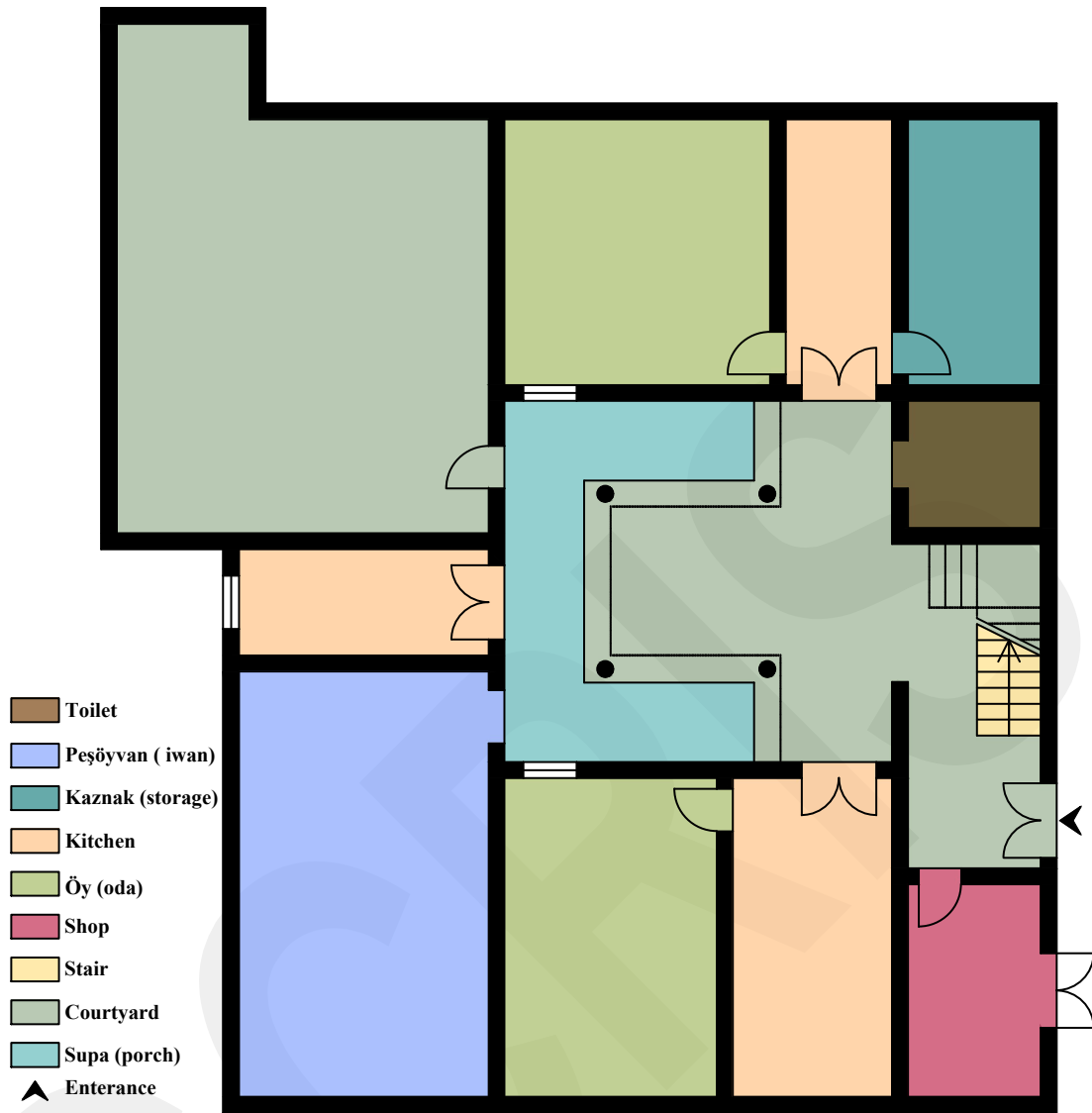
Figure 4.2.7 Plan of a eyvan-centered house in Kashgar Old City (source: Aibi, 2016)
