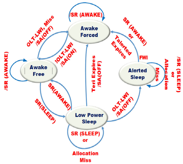
Fig. 3 Cyclic sleep state diagram for OLT
